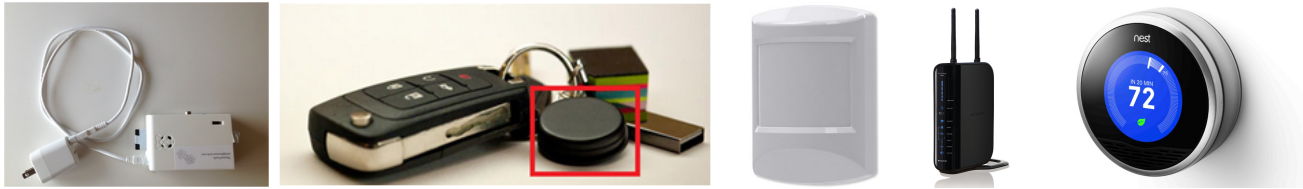
Figure 1: The hardware kit that was installed into each home included up to 4 data collection endpoints, up to 4 BLE tags, up to 6 motion sensors, 1 wireless router, and 1 Nest thermostat.
